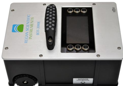
As of January 2014, this method replaces the old method for determining the static coefficient of friction in accordance with ASTM C1028 and is therefore the official method for determining the frictional resistance of hard flooring materials in the United States.
